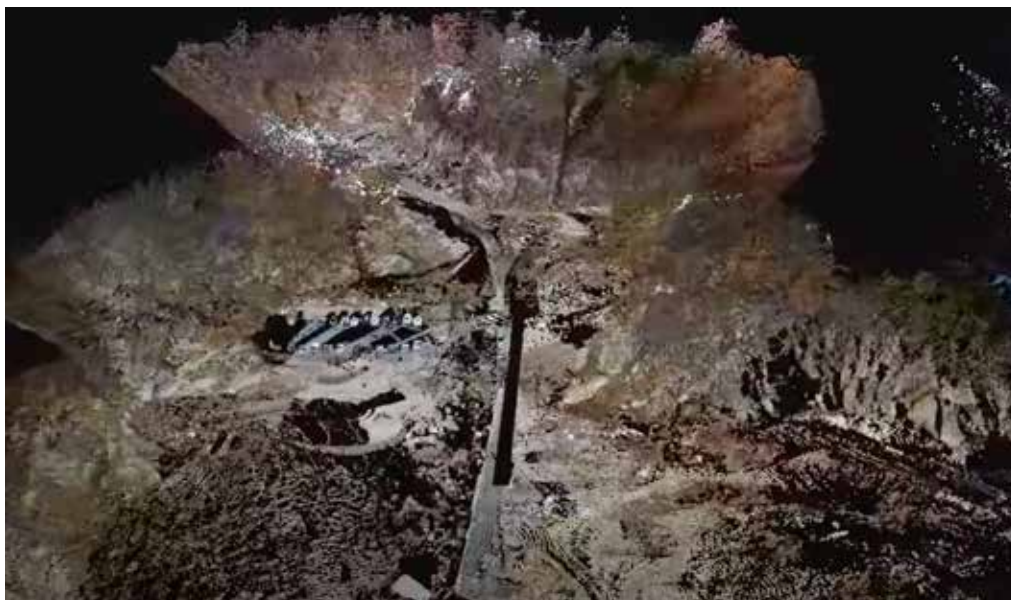
Precise surveying of tsunami-affected areas in the Aneyoshi district of Miyako City, Iwate Prefecture, using a terrestrial laser scanner
