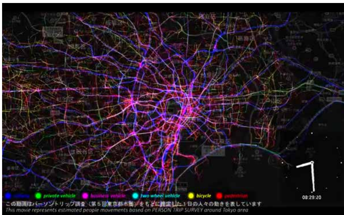
Visualization of People Flow data using person trip survey data (Tokyo metropolitan area, 2008)
