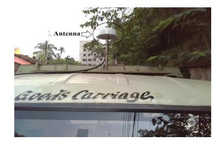
Pick up vehicle with external GNSS antenna
