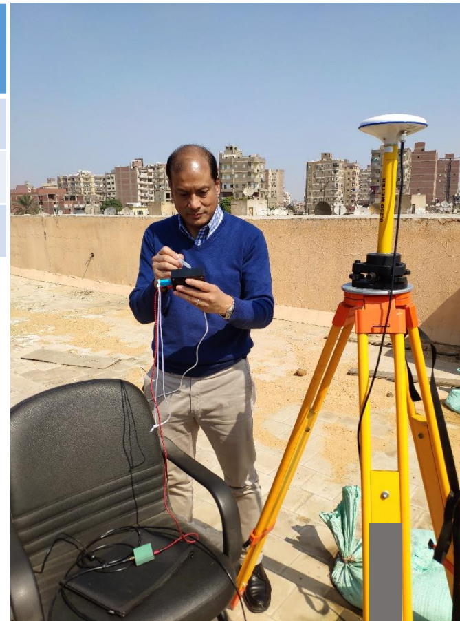
Setting MADOCA low-cost receiver system in RaspberryPi device.
