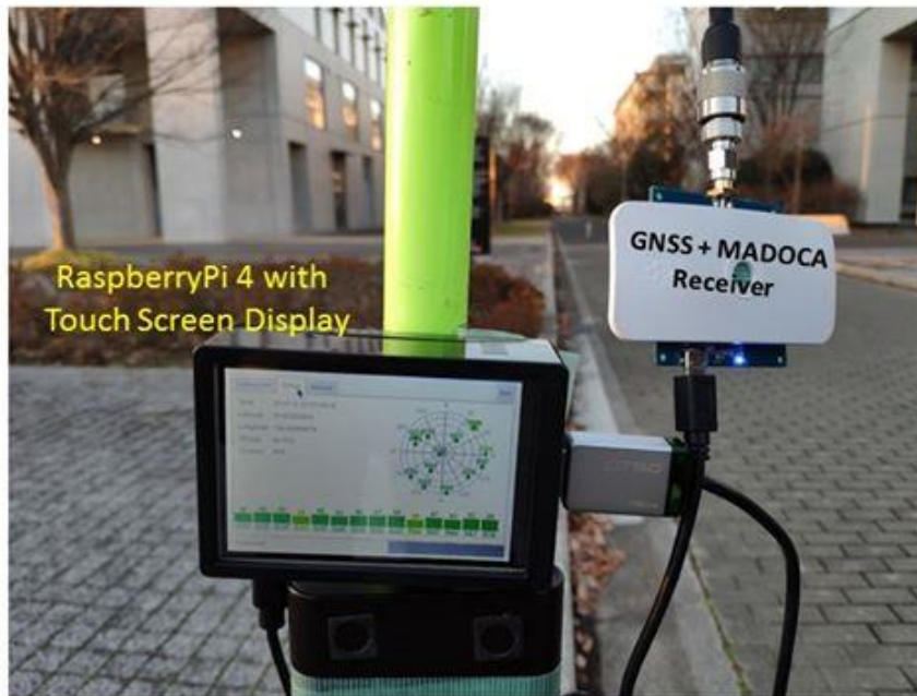
MADOCA PPP Receiver System based on RaspberryPi-4 Device
