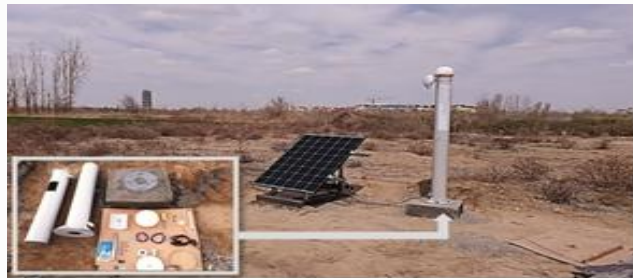
BDS integrated monitoring terminal Solar photovoltaic power supply system
