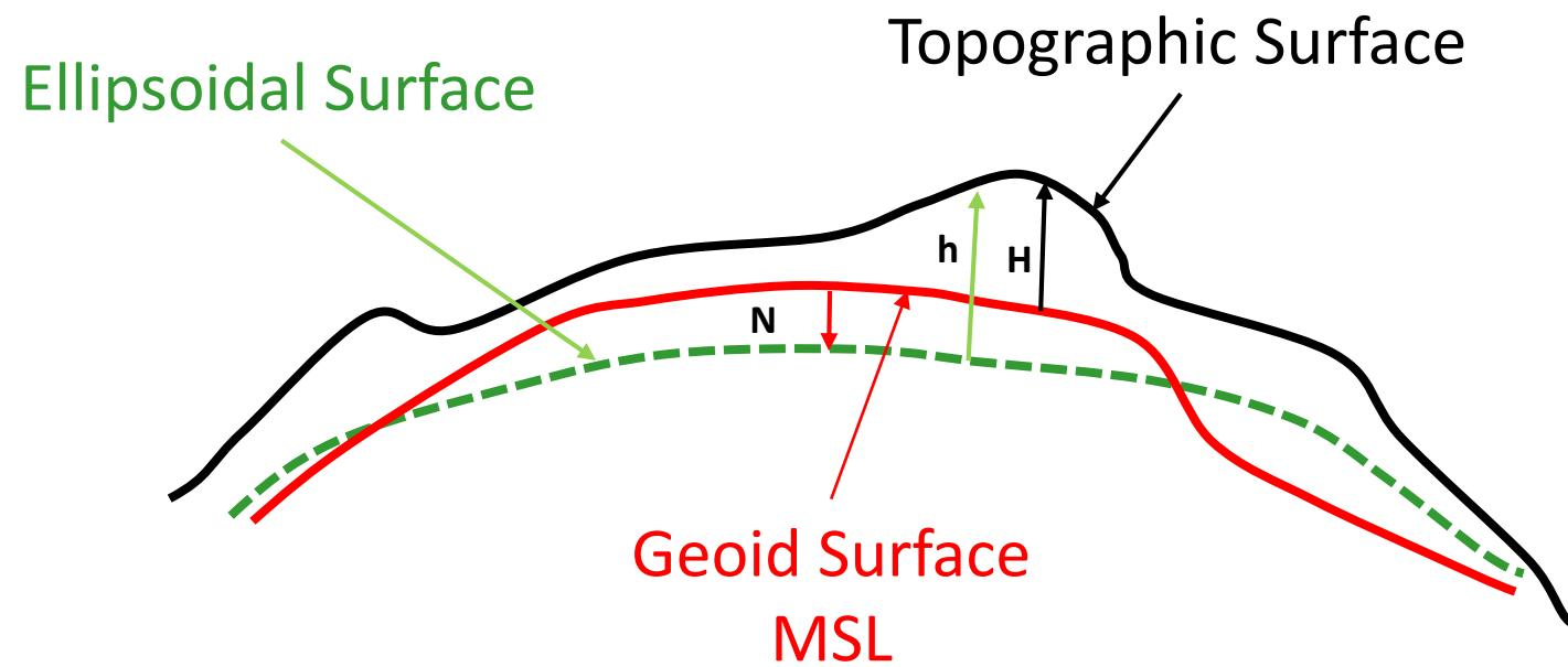
$$\text{Topographic Height (H)} = \text{Ellipsoidal Height (h)} - \text{Geoid Height (N)}$$
